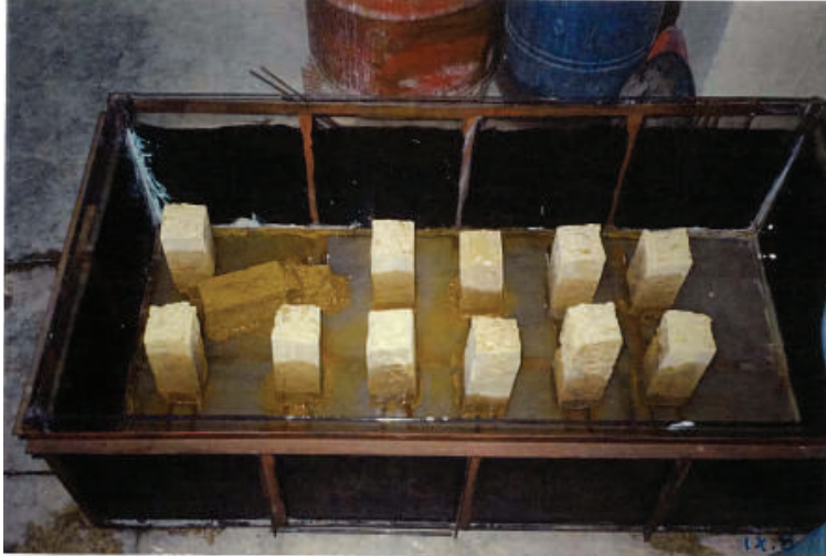
Resim 2.2. Kılcallık Deneyi Picture 2.2. Capillarity Experiment
