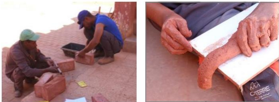
Figure 4: Photograph of a master builder rolling a moistened soil sample into a cylinder between their palms
