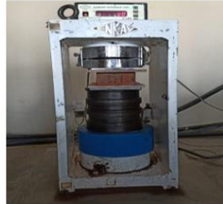
e) Compressive Strength Test of Bricks
