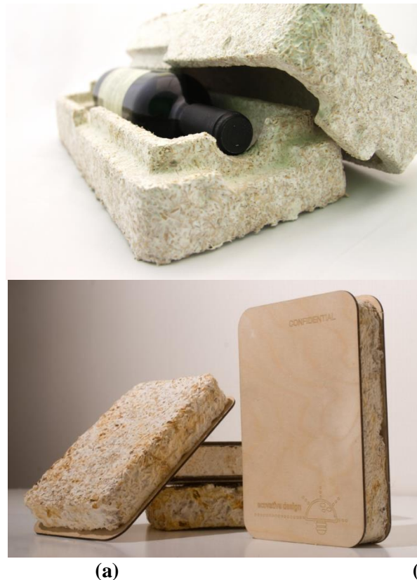
Image 3. Packaging foam (EcoCradle) produced by Ecovative company from buckwheat hulls and fungal mycelium (a) and insulation material (Greensulate) produced using agricultural by-products such as seed hulls and fungal mycelium as a binder (b) [25]
