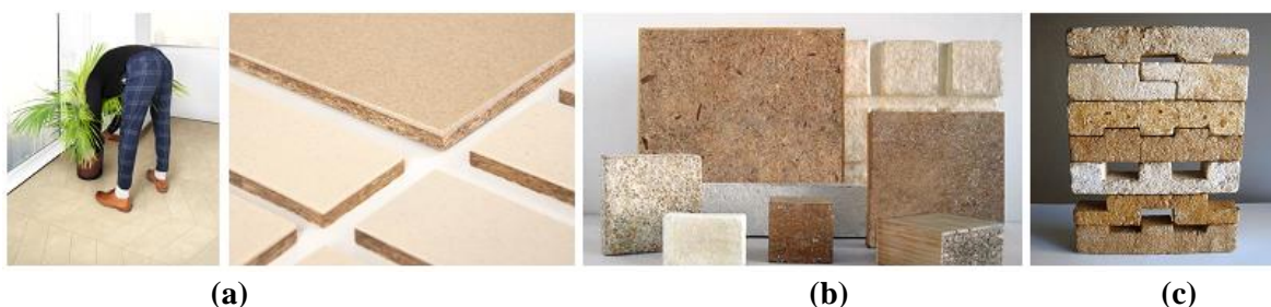
Image 4. Mycelium floor covering produced from selected fungal mycelium, cotton residues and low-value biomasses such as corn crops, rice straw, used coffee grounds, discarded seaweed and clam shells (a) [26], examples of various mycelium-based panel products (b) [27], examples of mycelium bricks (c) [28]
