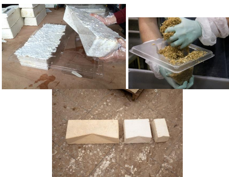
Image 8. Mycelium bricks grown from shredded corn stalks and mushroom mycelium [31]
