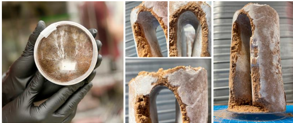
Image 14. Mycelium growing in regolith-like sand structures on Mars [38]
