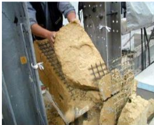
Figure 12: Geo-grid providing horizontal movement of the wall [16, 17].
