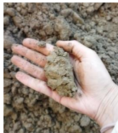
Figure 2. Soaked and Palm-integrated ALKER Sample, Source: E. Nurçin Kara Archive
