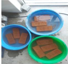
d) Water Absorption Test of Bricks
