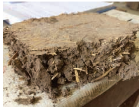
Figure 20. The brick made of palm frond after reaching the max. pressure (authors).
