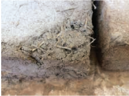
Figure 16. A sample made of 2(mud+sand) to 1 palm frond mixed by water (authors).
