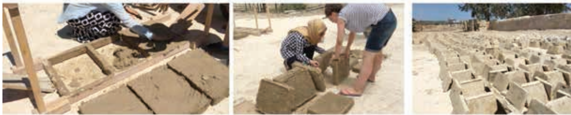
Figure 5. Removing the Adobe from the Moulds, Drying the Adobe (G. Benli archive, 2016)
