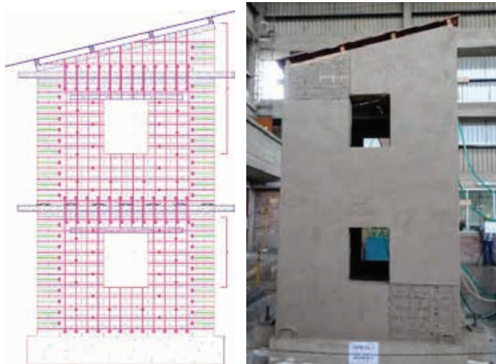
Figure 8. Two-story half-scale adobe reinforced model. Left: construction schematics. Right: test model on the shaking table.
