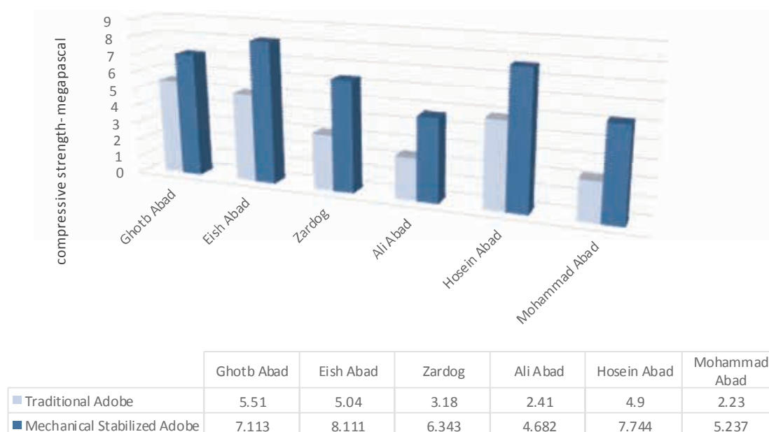
Figure 4. Comparison of the compression resistance of UA and SA.
