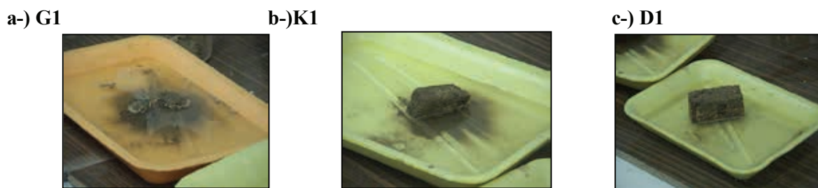
Figure 8. G1, K1, D1 Water Absorption of Samples by Capillarity
