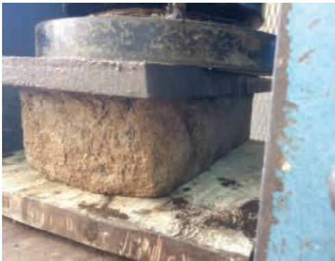
Figure 18. Testing the brick durability and strength (authors).
