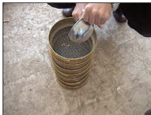
Figure 7. Sieving the Sample
