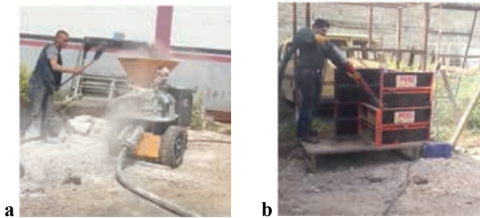
Figure 11 a, b. Machine mixed soil is (a) sprayed (b) and placed into molds.
