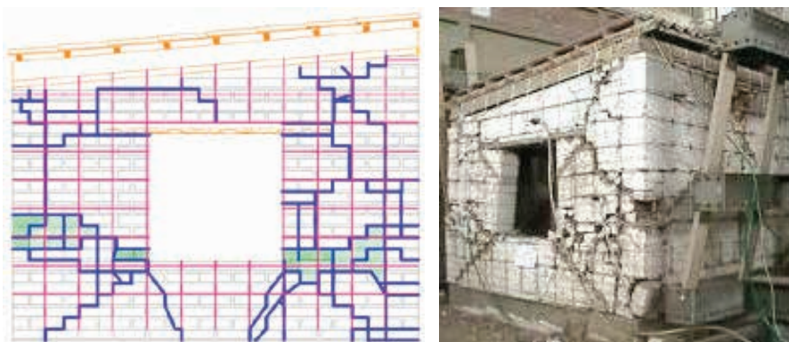
Figure 4. Repaired and reinforced adobe model after testing. Left: cracking pattern. Right: model after intense shaking table test.
