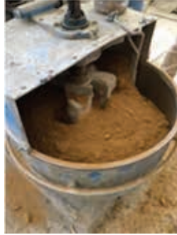
Figure 9. Using a cement mixer to mix the soil to be used in adobe production
