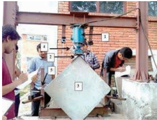
Figure 3. Test instrumentation setup; 1- hydraulic jack, 2- loading shoe, 3- test sample, 4- vertical displacement dial gauge, 5- horizontal displacement dial gauge
