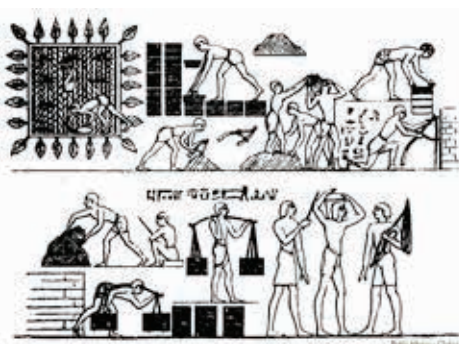
Figure 4. Ancient mural illustrates the ancient Egyptians method of mixing and building mud (url-3)
