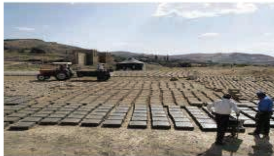
Figure 11. Drying adobe blocks
