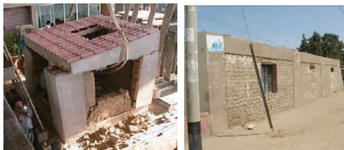
Figure 2. Adobe buildings with wire mesh reinforcement. Left: Brittle failure during test. Right: Undamaged house after 2007 earthquake.
