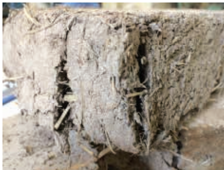
Figure 20. The brick made of palm frond after reaching the max. pressure (authors).
