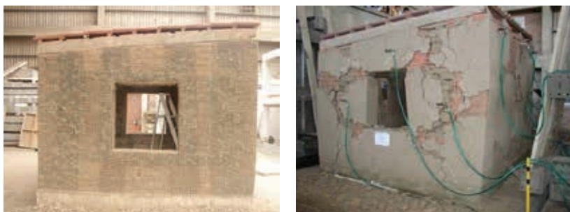
Figure 3. Adobe models reinforced with polymer mesh. Left: Geogrid. Right: Plastic mesh.
