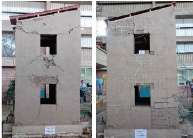
Figure 9. Two-story scaled models after shaking table testing. Left: unreinforced, close to collapse. Right: reinforced, with moderate damage.
