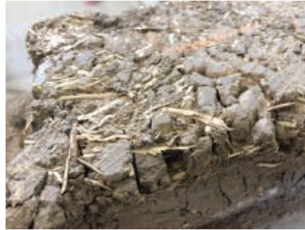
Figure 16. A sample made of 2(mud+sand) to 1 palm frond mixed by water (authors).
